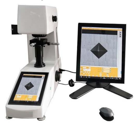
PCHVT-1000Z is a new generation of Micro Vickers hardness tester adopts the integrated design of hardness tester and panel computer, all the testing parameters can be selected on the panel computer.
